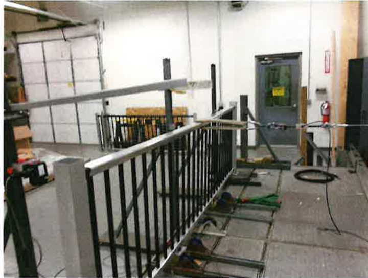
Photo No. 3 Horizontal Concentrated Load Test at Midspan of Top Rail
