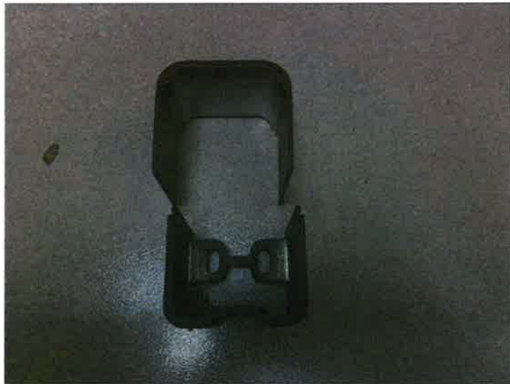
Photo No. 12 Cast Aluminum Bracket for Bottom Rail
