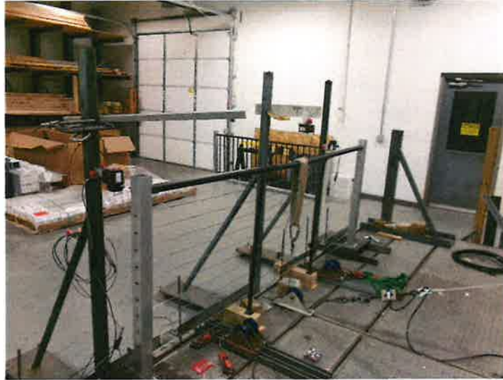
Photo No. 7 Vertical Concentrated Load Test at Midspan of Top Rail
