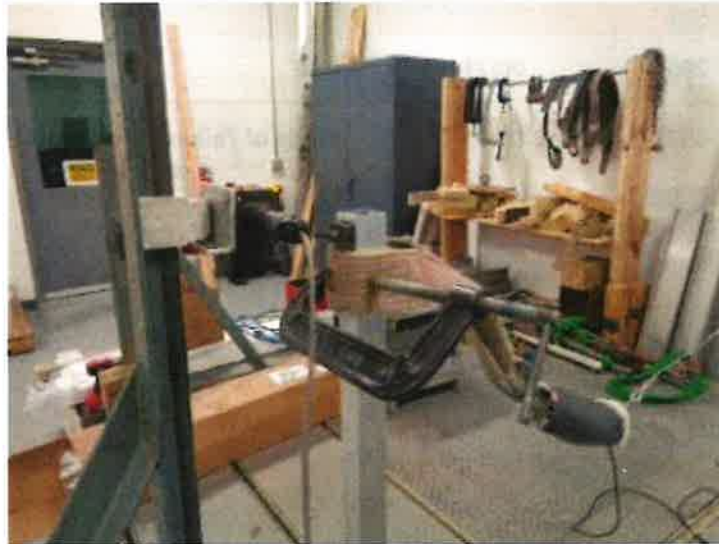
Photo No. 1 Static Post Load Test
