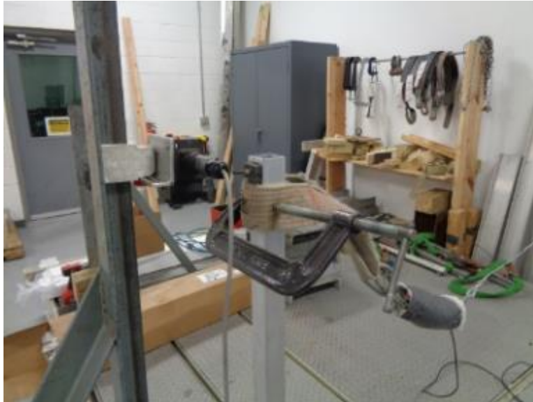
Photo No. 1 Static Post Load Test
