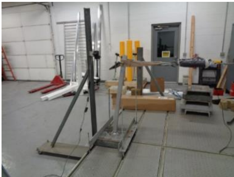
Photo No. 2 Static Post Load Test - Load Applied
