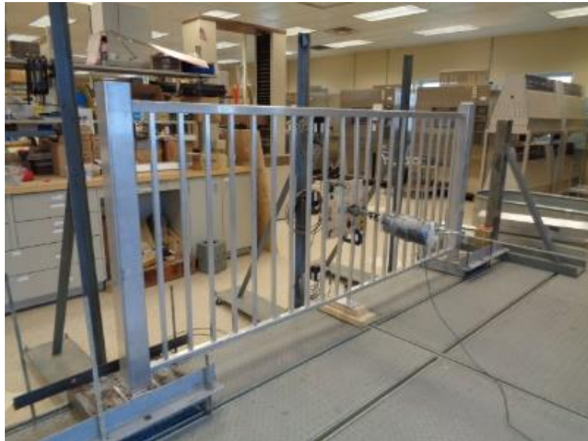
Photo No. 1 In-Fill Load Test at Center of Two Pickets
