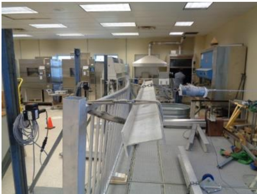
Photo No. 4 Concentrated Load at Ends of Rail (Brackets)
