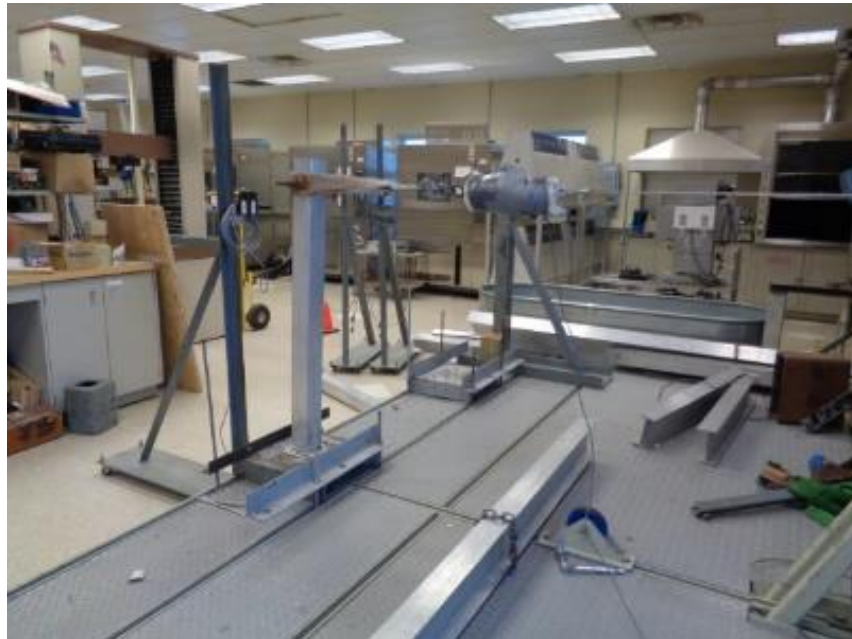
Photo No. 5 Concentrated Load Test at Top of Post Mount
