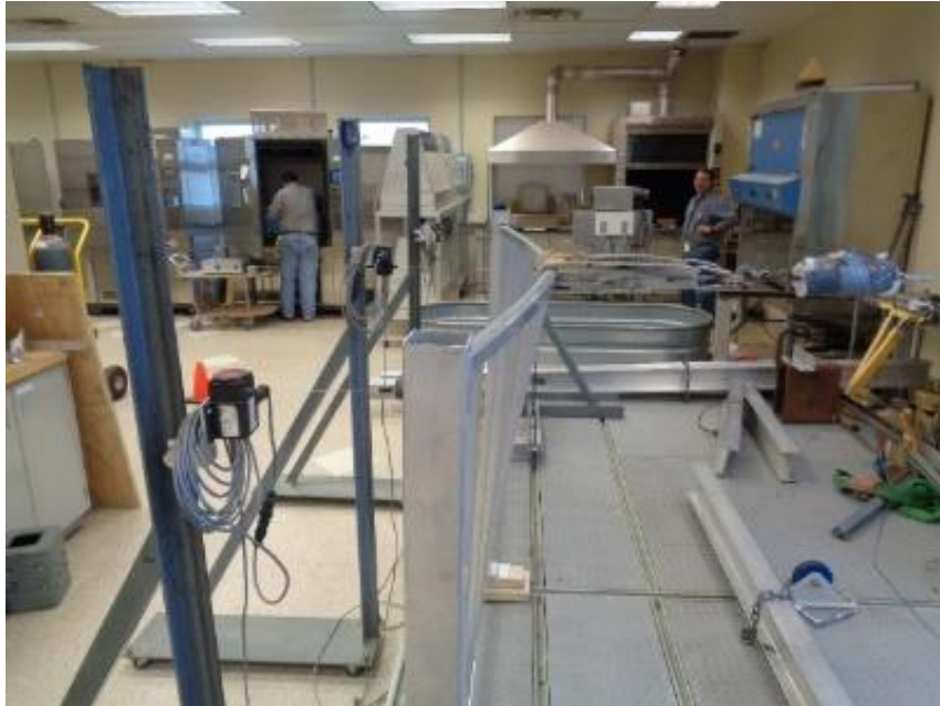
Photo No. 3 Concentrated Load Test at Mid-Span of Top Rail
