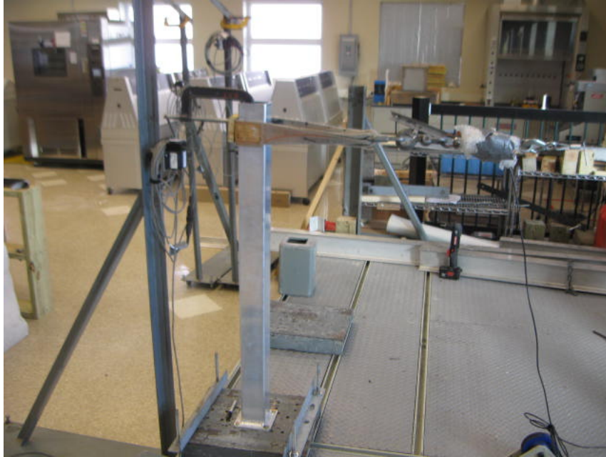
Photo No. 1 Horizontal Loading of aluminum post, surface-mounted on a steel channel
