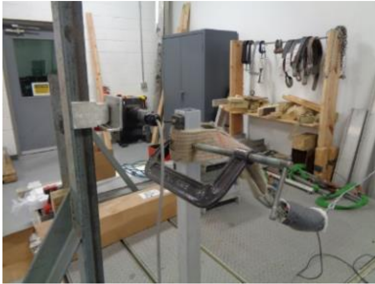
Photo No. 1 Static Post Load Test
